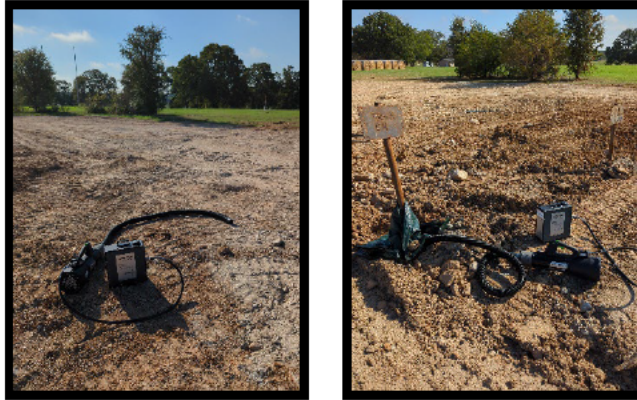
Figure 10: Photos showing methane emissions quantification with the Hi-Flow 2 gathering background data (left) and leak test data (right) at the B-5H.
